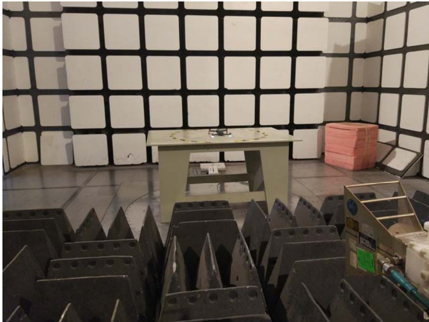
Radiated Emissions View (Above 1 GHz, Playing)
