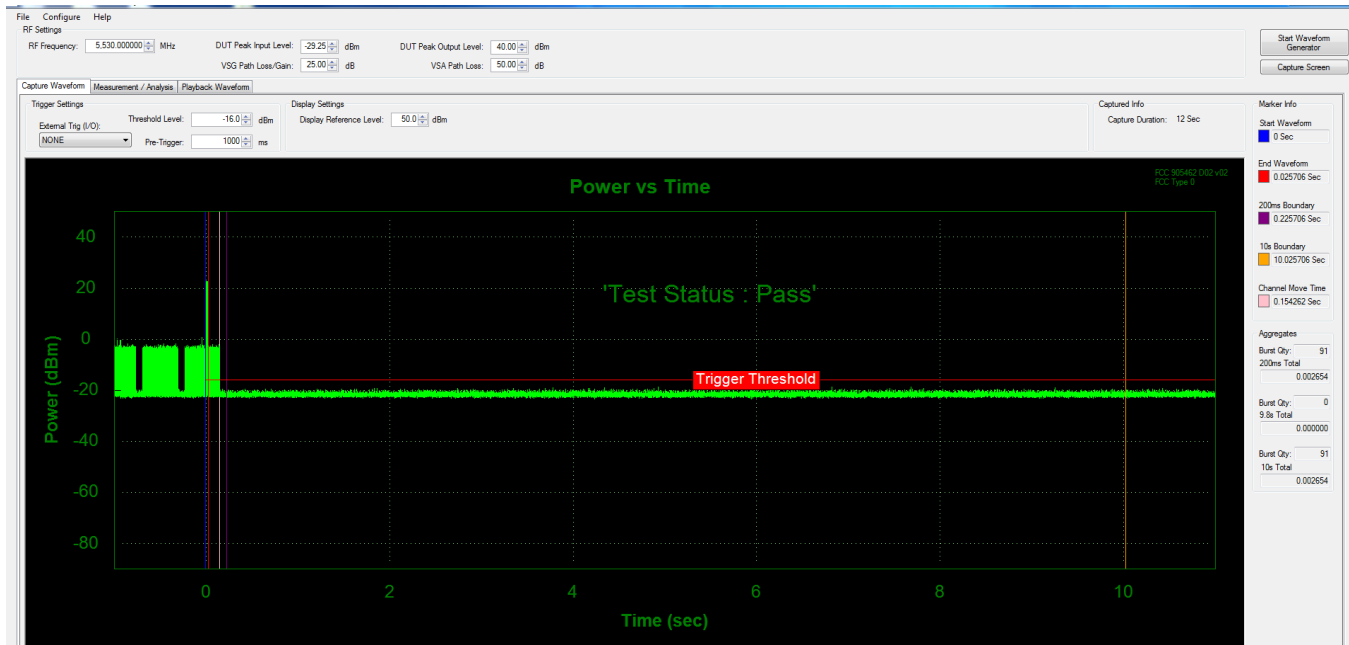
Figure 9-33. 5530MHz - Channel Move/ Closing Transmission Time - Mode 3 (80 MHz)
