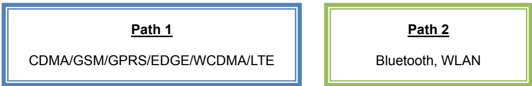
Figure 13.1 Simultaneous Transmission Paths
