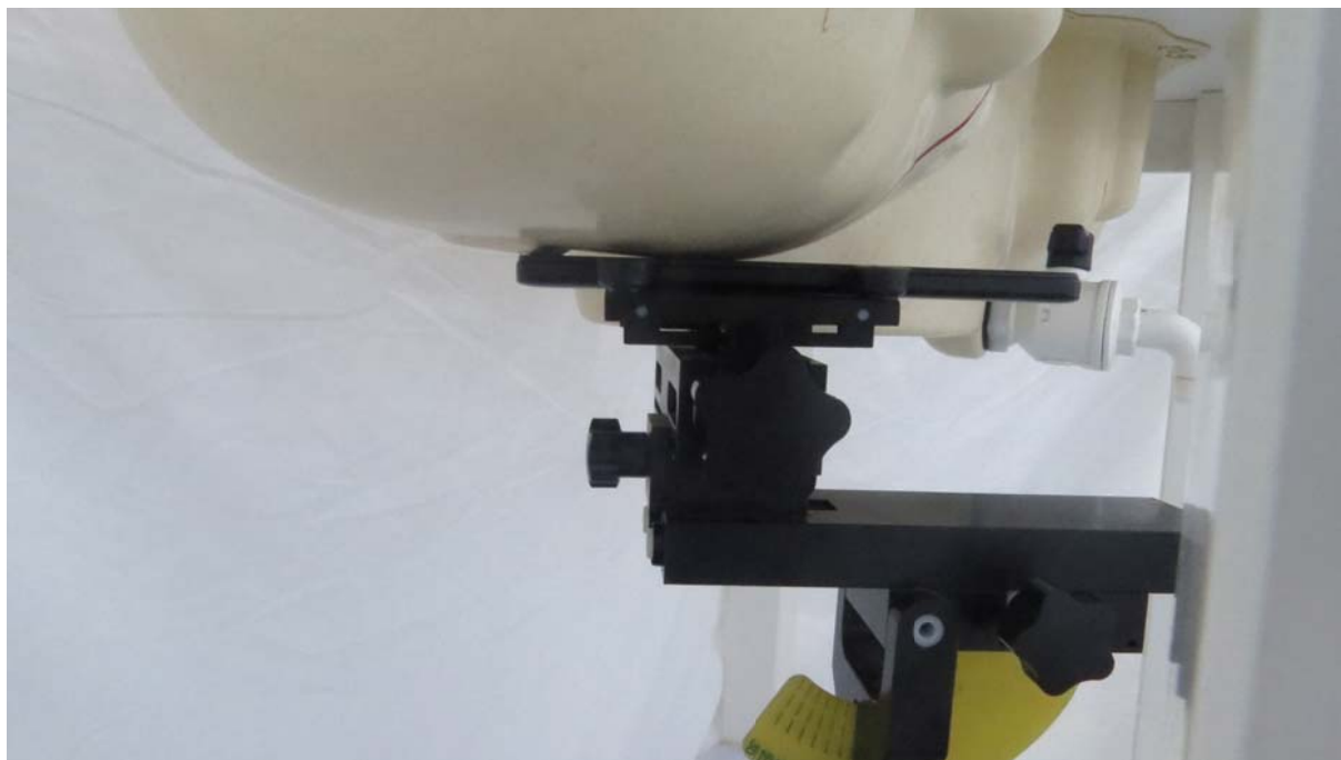
Picture 3: Right Hand Touch Cheek Position
