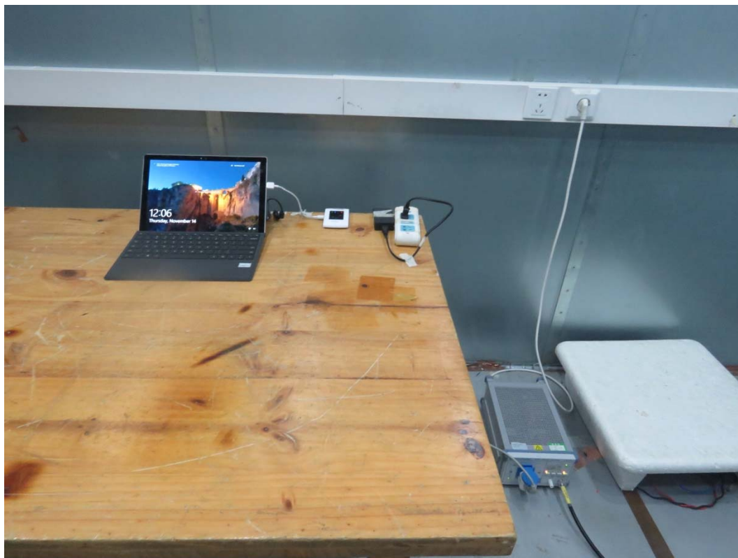
Picture 2 Conducted Emission Test Setup
