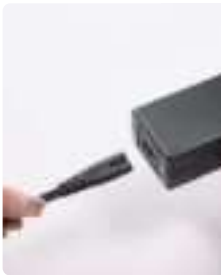
3. Connect the power cord and plug in the power supply
