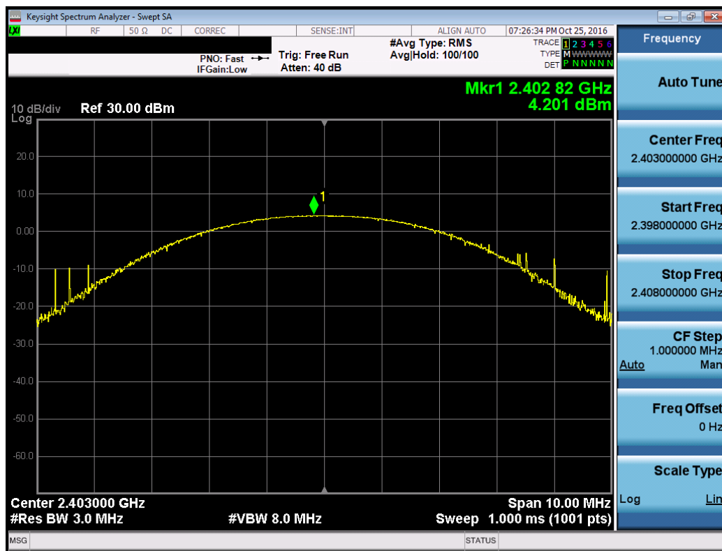
Plot 7-13. Peak Conducted Power (EX600-WEN3-X40, Ch. 0)
