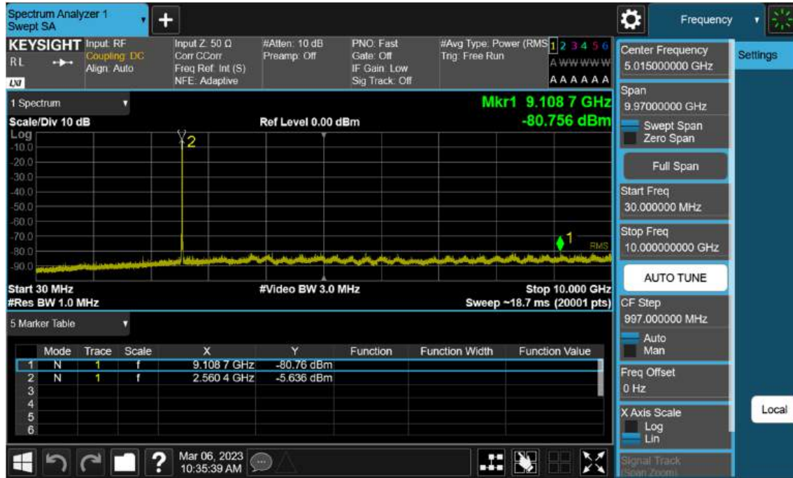
Sub6 n7. Conducted Spurious_1 (513000ch_10 MHz_BPSK_RB 1)
