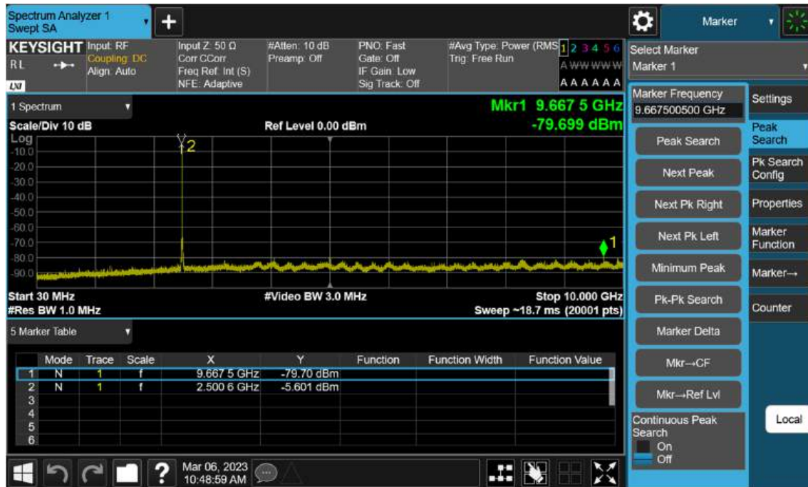
Sub6 n7. Conducted Spurious_1 (502000ch_20 MHz_BPSK_RB 1)
