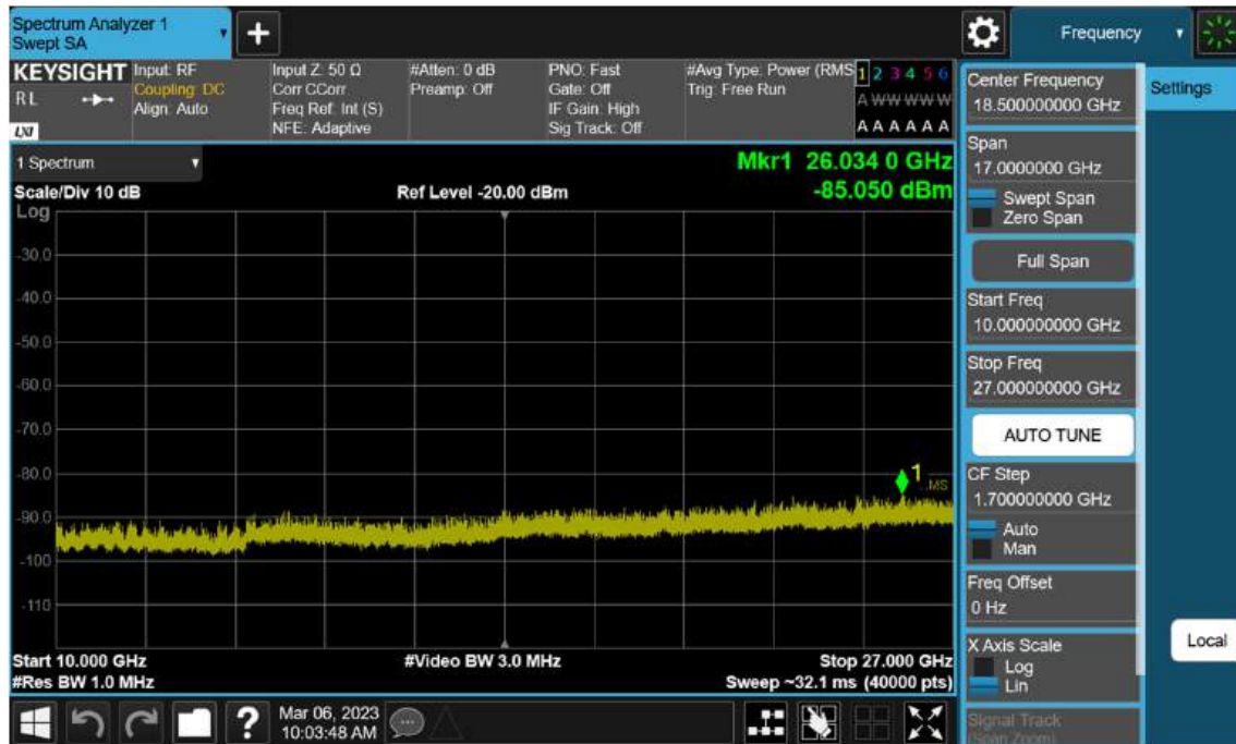
Sub6 n7. Conducted Spurious_2 (507000ch_5 MHz_BPSK_RB 1)
