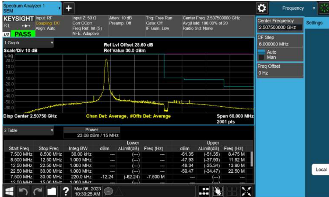
Sub6 n7. Low Channel Edge Plot (15 MHz Ch.501500 BPSK_RB1)-2
