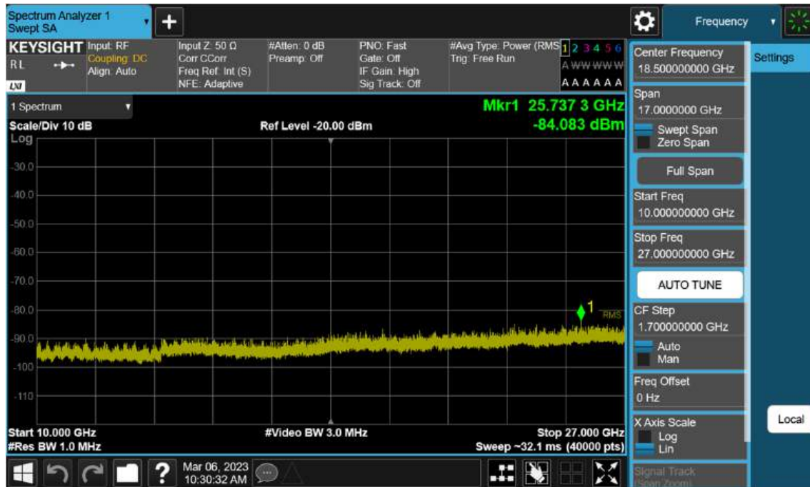
Sub6 n7. Conducted Spurious_2 (501000ch_10 MHz_BPSK_RB 1)
