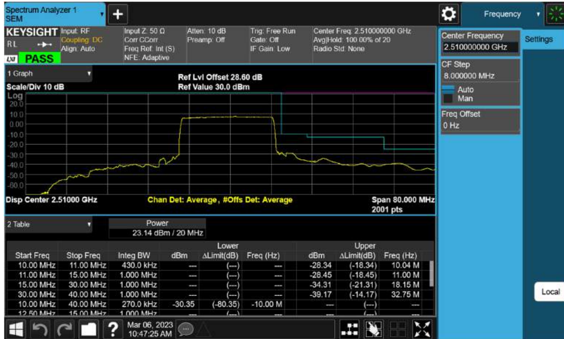
Sub6 n7. Low Channel Edge Plot (20 MHz Ch.502000 BPSK)-2
