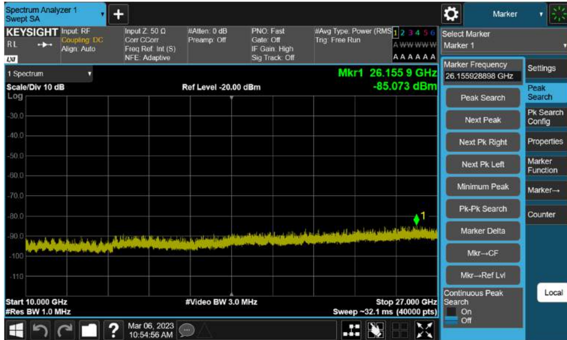
Sub6 n7. Conducted Spurious_2 (512000ch_20 MHz_BPSK_RB 1)
