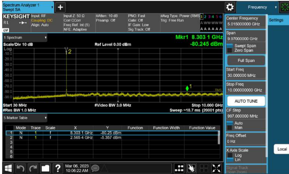
Sub6 n7. Conducted Spurious_1 (513500ch_5 MHz_BPSK_RB 1)
