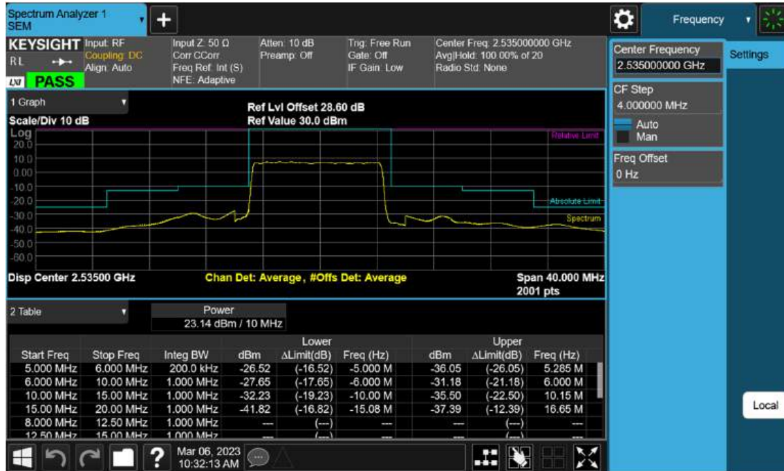
Sub6 n7. Mid Channel Edge Plot (10 MHz Ch.507000 BPSK)
