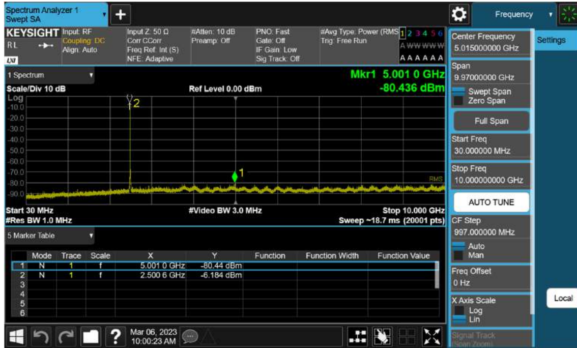
Sub6 n7. Conducted Spurious_1 (500500ch_5 MHz_BPSK_RB 1)
