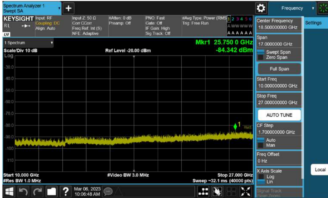
Sub6 n7. Conducted Spurious_2 (513500ch_5 MHz_BPSK_RB 1)
