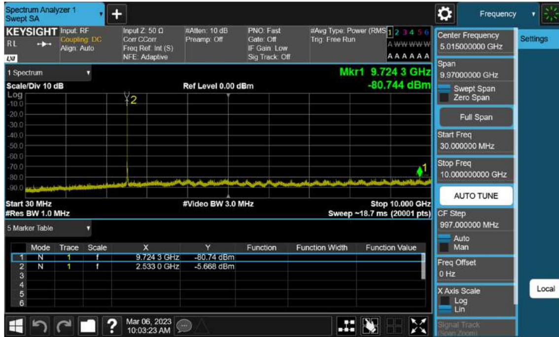
Sub6 n7. Conducted Spurious_1 (507000ch_5 MHz_BPSK_RB 1)
