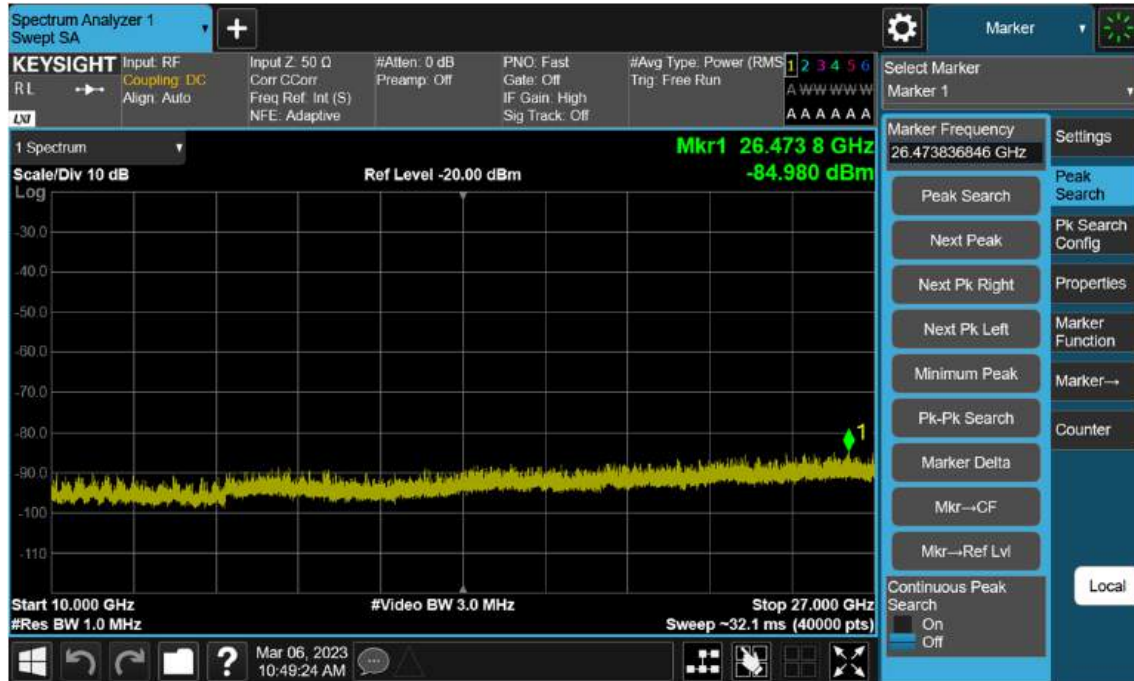
Sub6 n7. Conducted Spurious_2 (502000ch_20 MHz_BPSK_RB 1)
