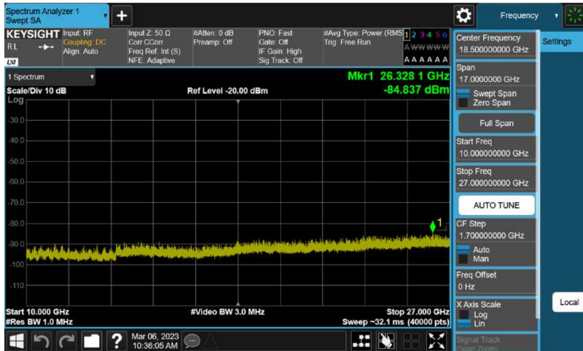
Sub6 n7. Conducted Spurious_2 (513000ch_10 MHz_BPSK_RB 1)
