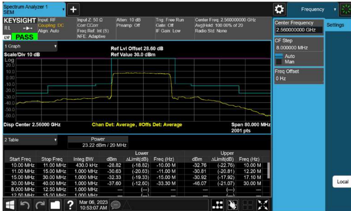
Sub6 n7. High Channel Edge Plot (20 MHz Ch.512000 BPSK)
