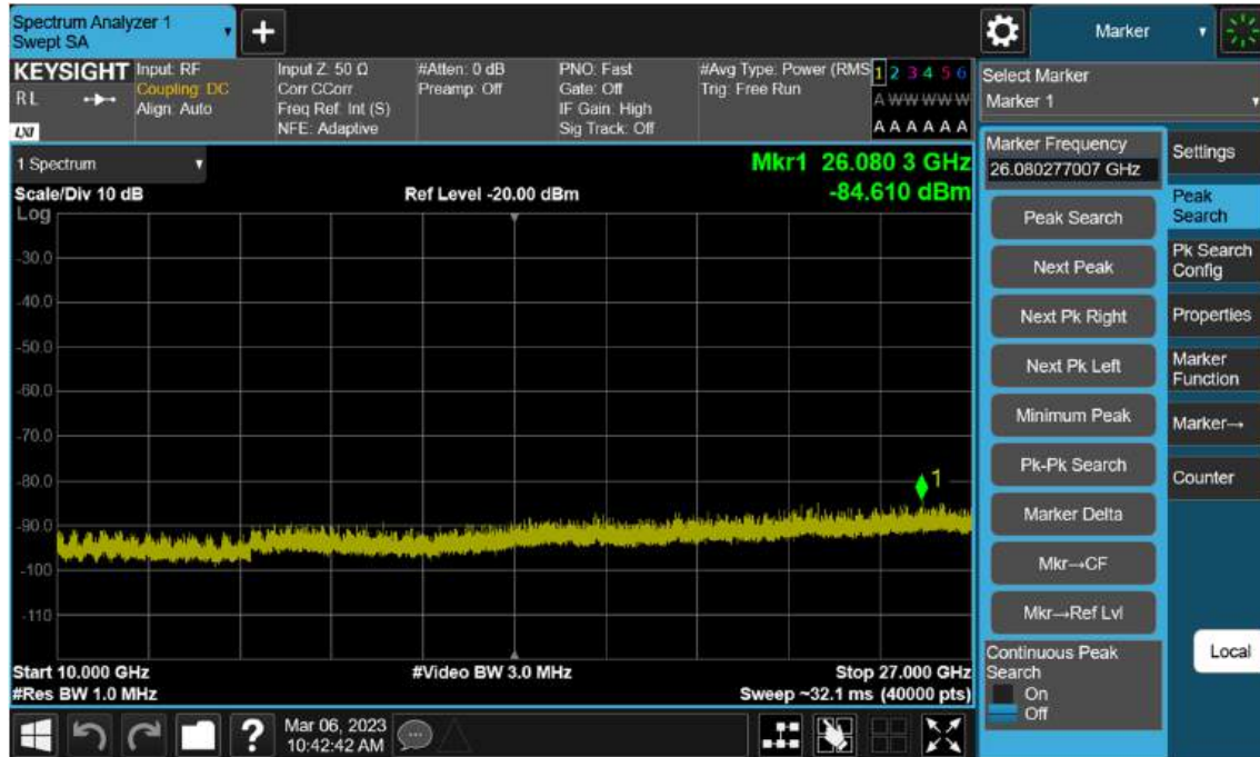
Sub6 n7. Conducted Spurious_2 (507000ch_15 MHz_BPSK_RB 1)
