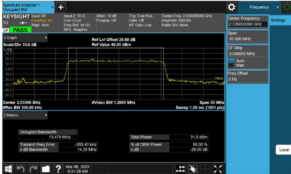
Sub6 n7. Occupied Bandwidth Plot (15 M BW Ch.507000 BPSK)
