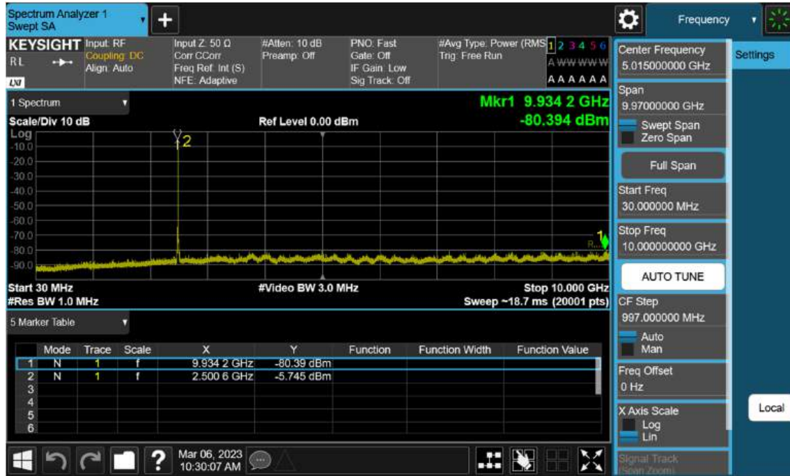
Sub6 n7. Conducted Spurious_1 (501000ch_10 MHz_BPSK_RB 1)
