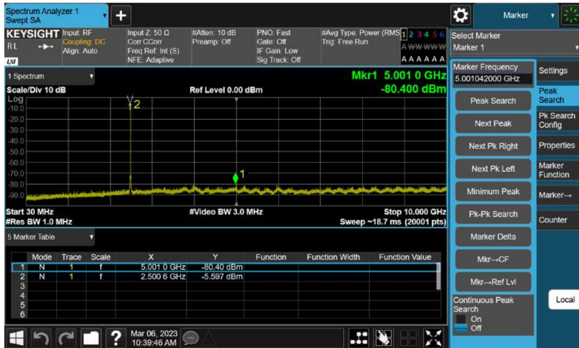
Sub6 n7. Conducted Spurious_1 (501500ch_15 MHz_BPSK_RB 1)
