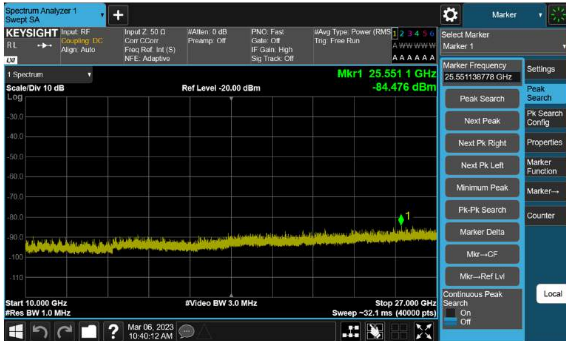
Sub6 n7. Conducted Spurious_2 (501500ch_15 MHz_BPSK_RB 1)
