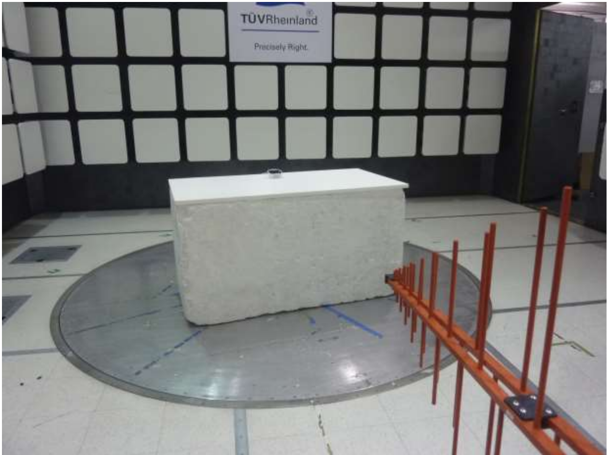
Figure 4: Test Setup for 30 MHz to 1 GHz (View 2)
