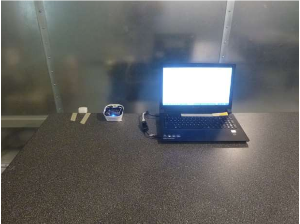
Figure 11: Conducted Emission Test Setup (Front)
