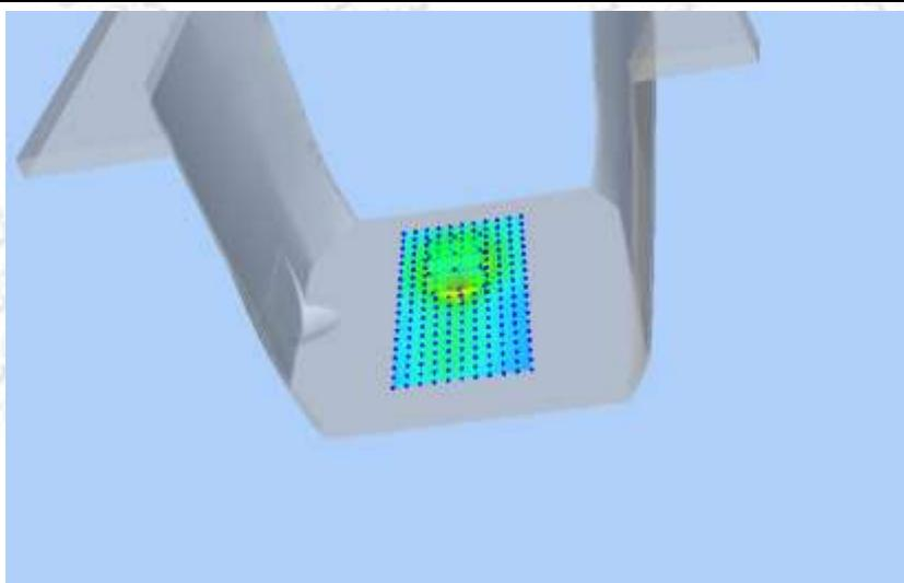
Test Mode:GPRS1900MHz, Mid channel(Body SAR-LCD Down)
