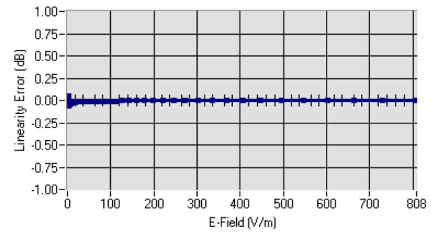
Linearity:  $\pm 1.47\%$  ( $\pm 0.06\text{dB}$ )5.3 SENSITIVITY IN LIQUID
