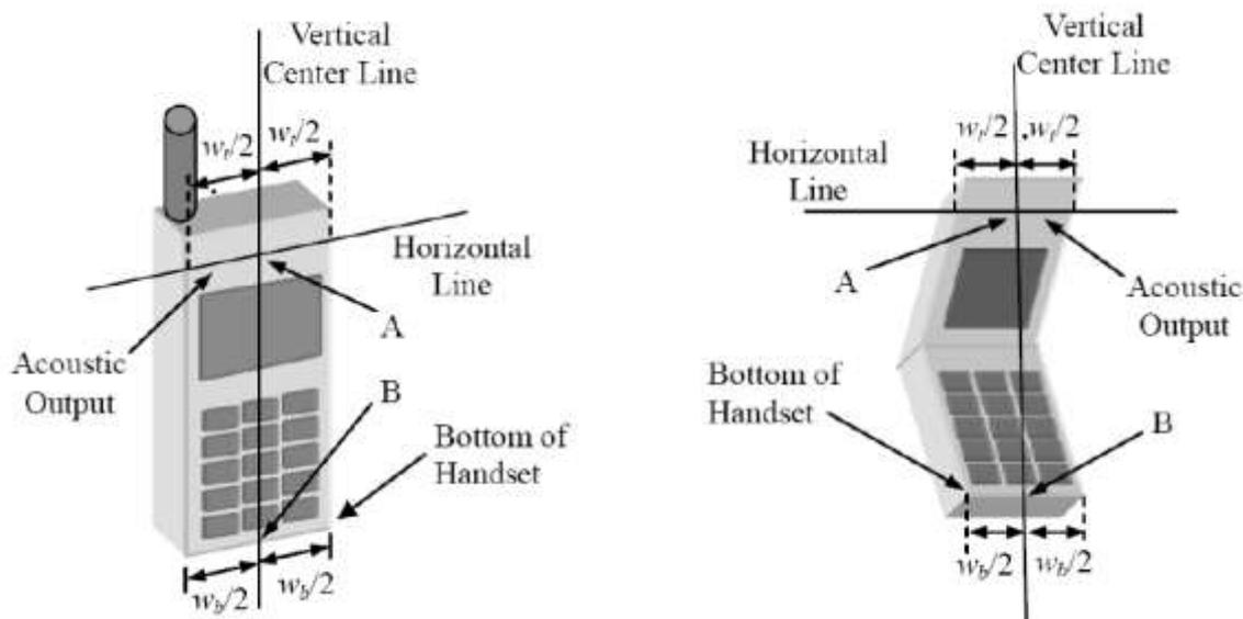
$W_r$  Width of the handset at the level of the acoustic
