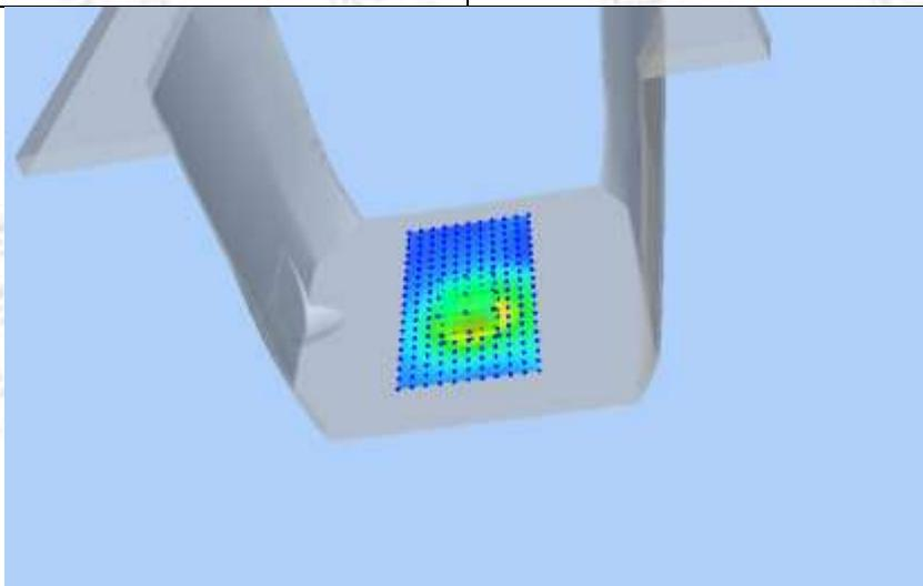
Test Mode:802.11b, Mid channel(Body SAR-LCD DOWN)
