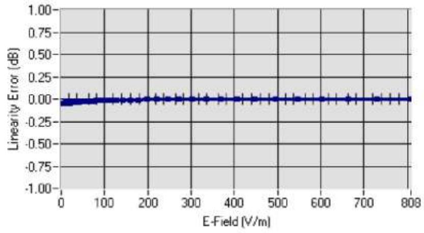
Linearity:  $\pm 1.16\%$  ( $\pm 0.05\text{dB}$ )5.3 SENSITIVITY IN LIQUID
