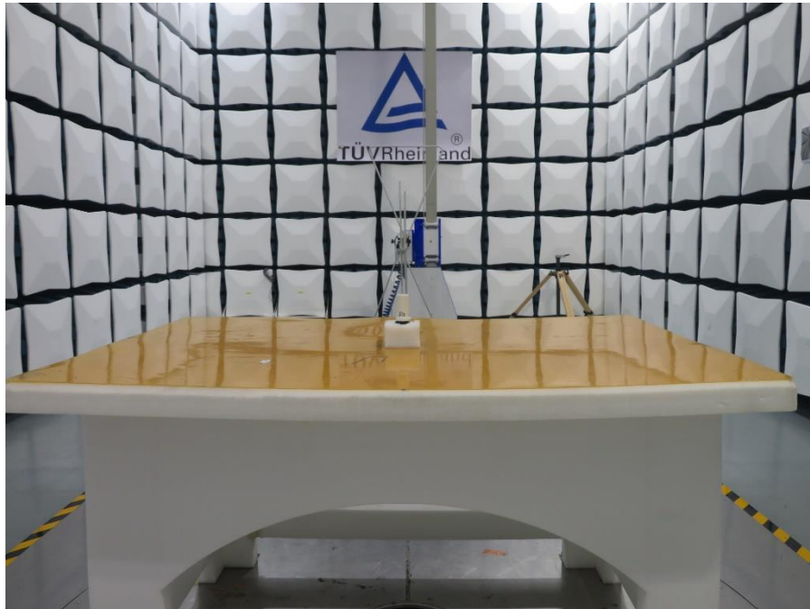
Photograph 1: Set-up for Radiated Spurious Emission, Below 1GHz
