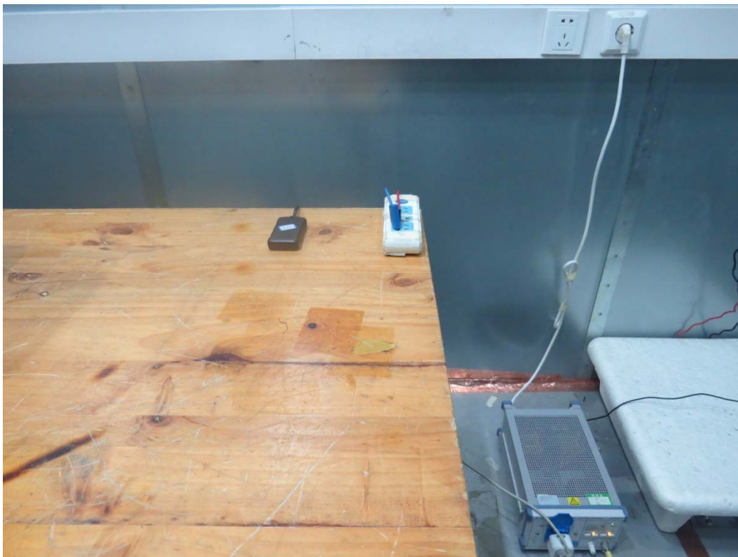
Picture 2 Conducted Emission Test Setup
