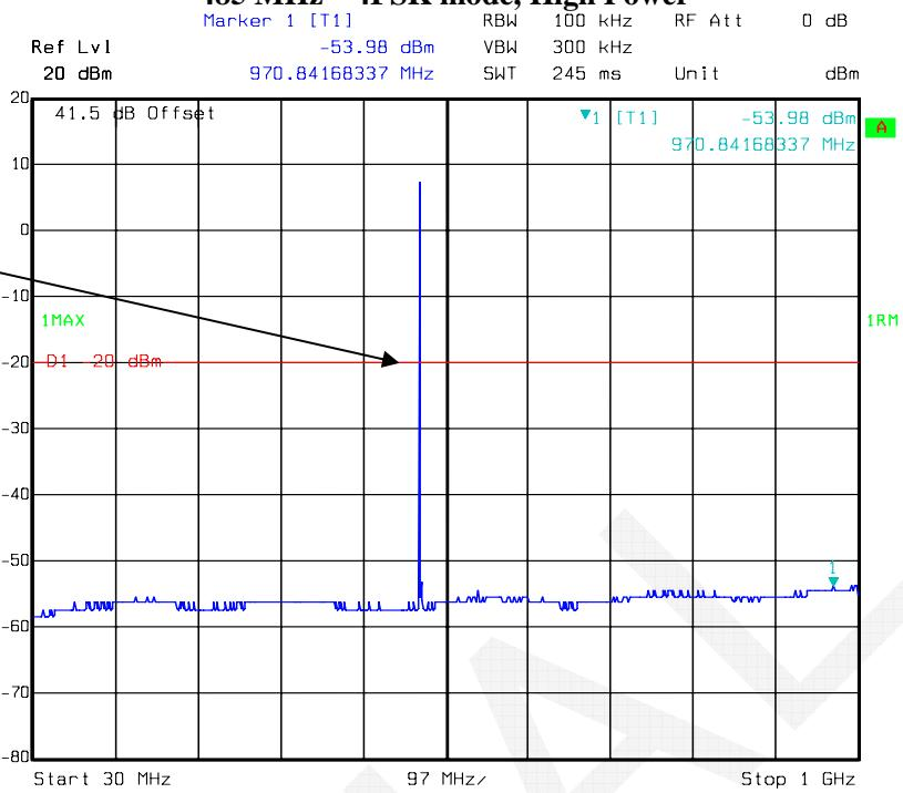
Fundamental test with Band Reject Filter
