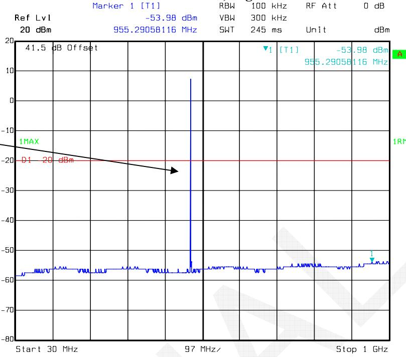
Fundamental test with Band Reject Filter
