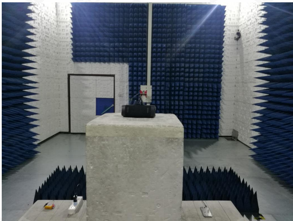
RADIATED EMISSION TEST SETUP ABOVE 1GHZ
