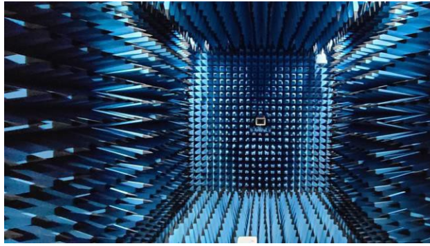
Figure 2: Geometry of Anechoic Chamber for Radiation patterns.
