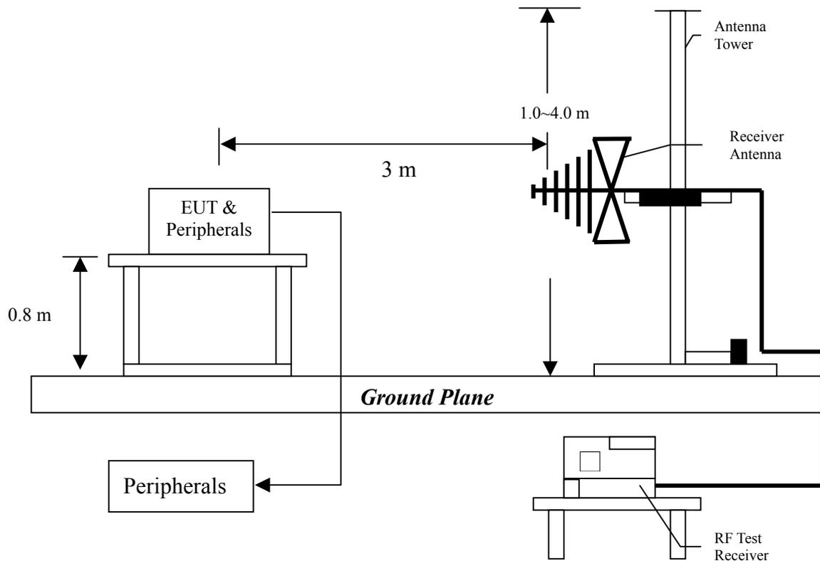
Radiated emissions were investigated cover the frequency range from 30MHz to 1000MHz using a receiver RBW of 120kHz record QP reading, and the frequency over 1GHz using a spectrum analyzer RBW of 1MHz and 10Hz VBW record Average reading. (15.209 paragraph), the Peak reading (1MHz RBW/VBW) recorded also on the report.
