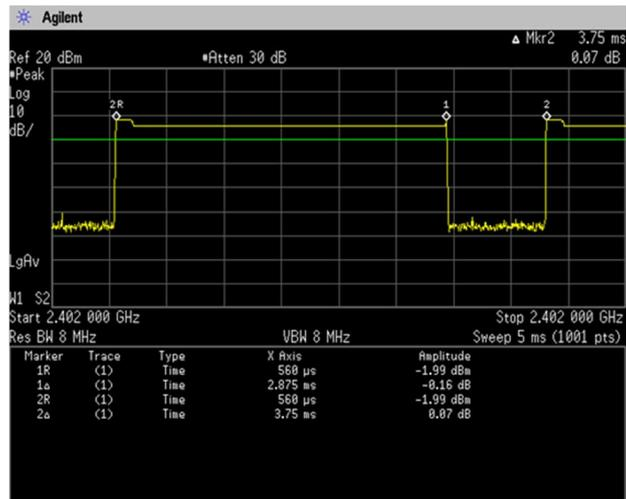
$$\text{Duty Cycle} = \text{Ton} / (\text{Ton} + \text{Toff}) = 2.875[\text{ms}] / (2.875[\text{ms}] + 0.875[\text{ms}]) = 76.67[\%]$$
