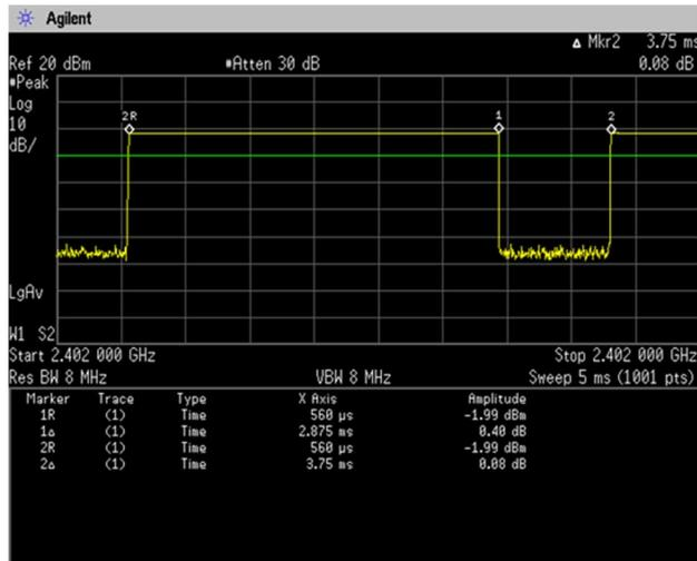
$$\text{Duty Cycle} = \text{Ton} / (\text{Ton} + \text{Toff}) = 2.875[\text{ms}] / (2.875[\text{ms}] + 0.875[\text{ms}]) = 76.67[\%]$$
