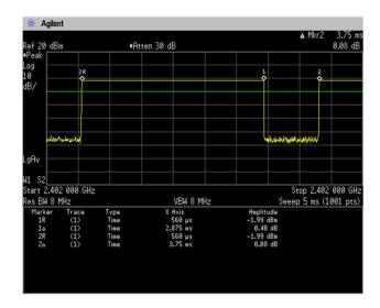
Duty Cycle = Ton / (Ton + Toff) = 2.875[ms] / (2.875[ms] + 0.875[ms]) = 76.67[%]
