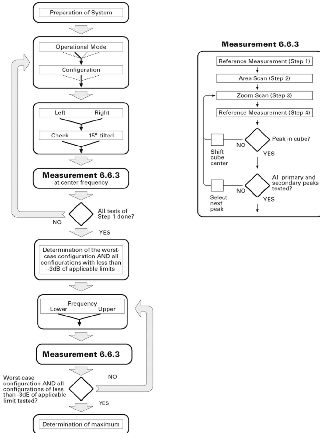
Establish a call with the maximum output power with a base station simulator, the connection between the EUT and the base station simulator is established via air interface.
