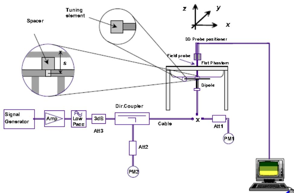
With the SG and Amp and with directional coupler in place, set up the source signal at the relevant frequency and use a power meter to measure the power at the end of the SMA cable that you intend to connect to the balanced dipole. Adjust the SG to make this, say, 0.25W (24 dBm). If this level is too high to read directly with the power meter sensor, insert a calibrated attenuator (e.g. 10 or 20 dB) and make a suitable correction to the power meter reading.
