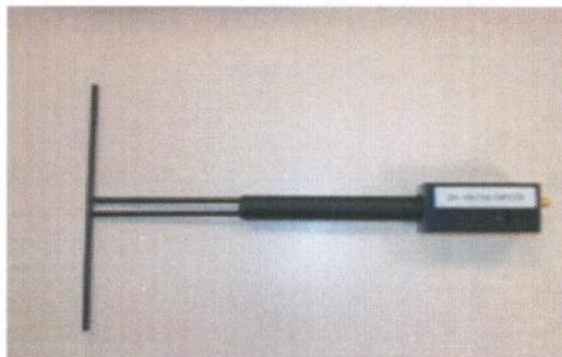
**Figure 1 – Satimo COMOSAR Validation Dipole**
