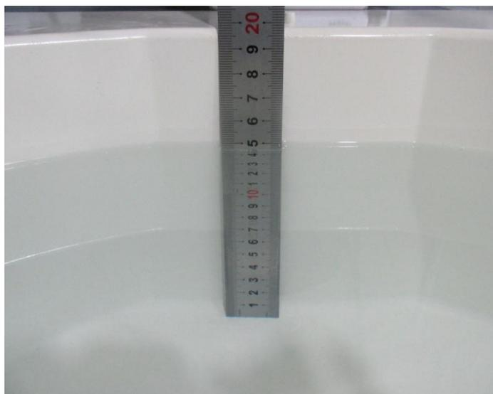
**Fig.9 Body Liquid of 1900MHz(15cm)**
