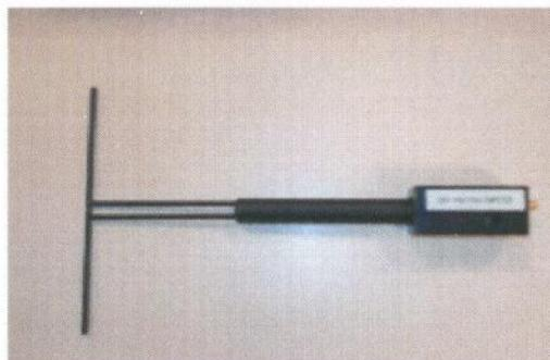
**Figure 1 – Satimo COMOSAR Validation Dipole**
