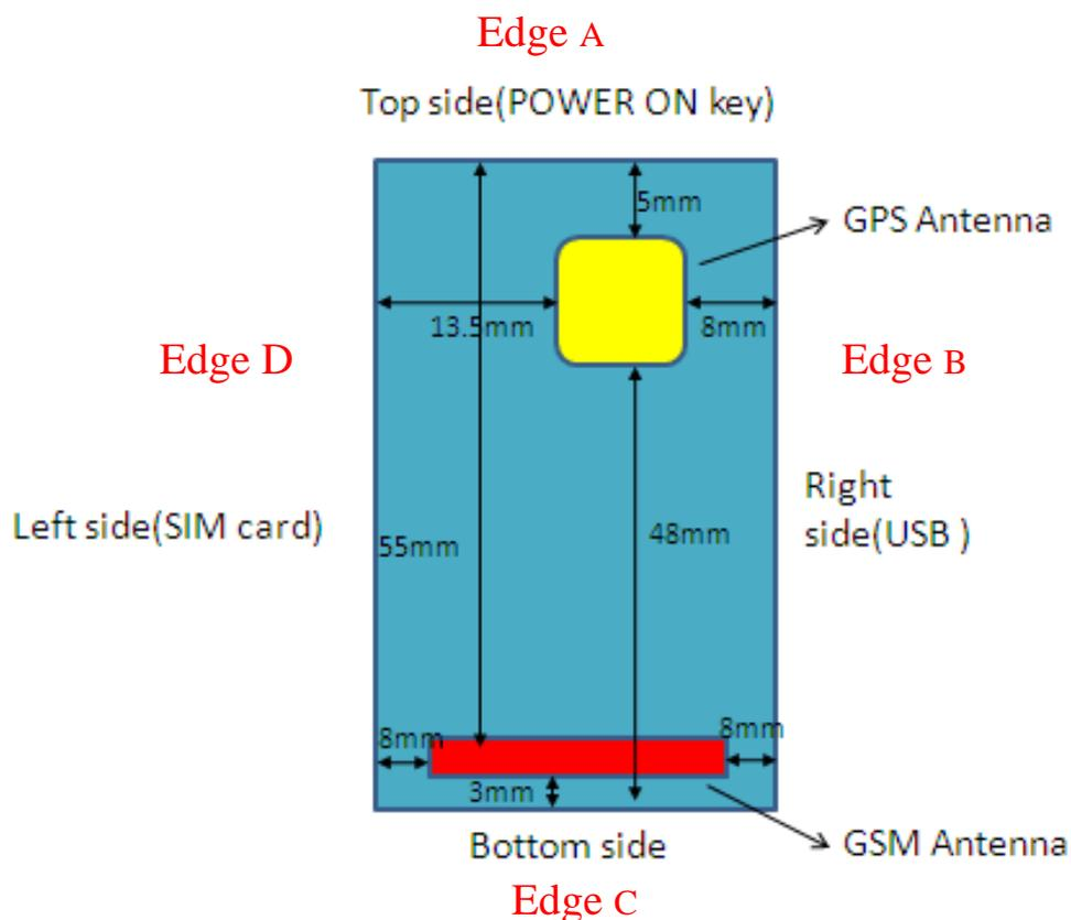
Fig. 3 Position of the antennas
