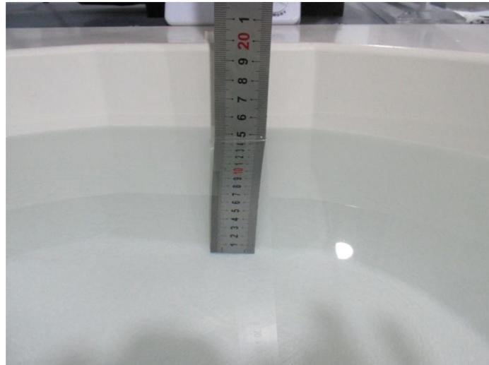
**Fig.8 Body Liquid of 835MHz(15cm)**
