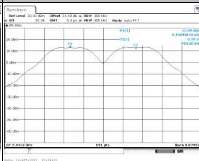
Channel Separation Plot on Channel 39 - 40
