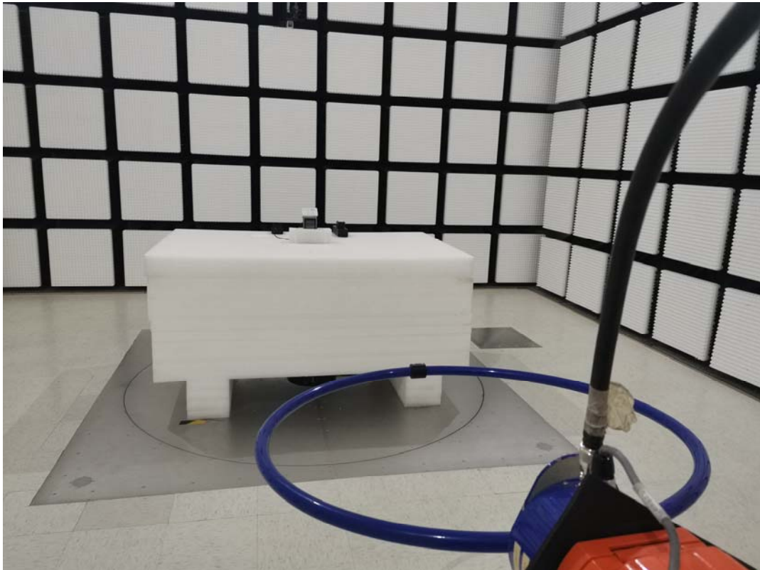
Radiated Emission Below 1G View
