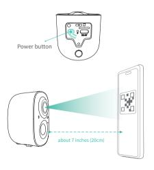
3) After a while, the camera will give out a prompt sound of a successful connection. At this moment, please set the name for the device on the App and select the location you want to place the device. Click "Continue" to complete the pairing.
