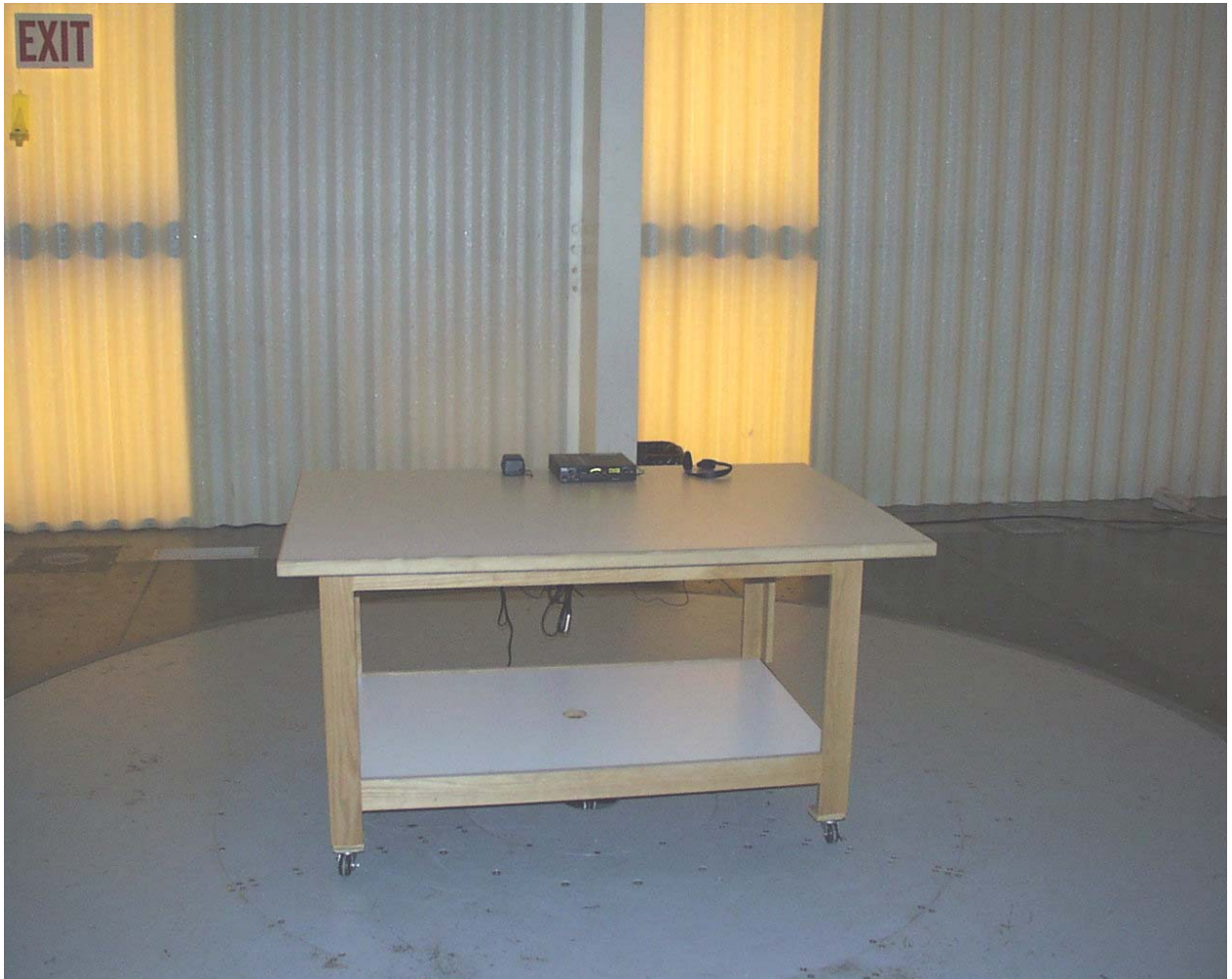
Front View Radiated Spurious Emission Configuration
