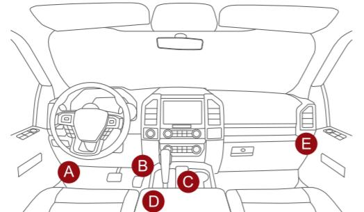
Usually, the OBDII port is located under the dashboard, above the pedal on the driver's side. The five locations shown in the picture are common OBDII port locations.
