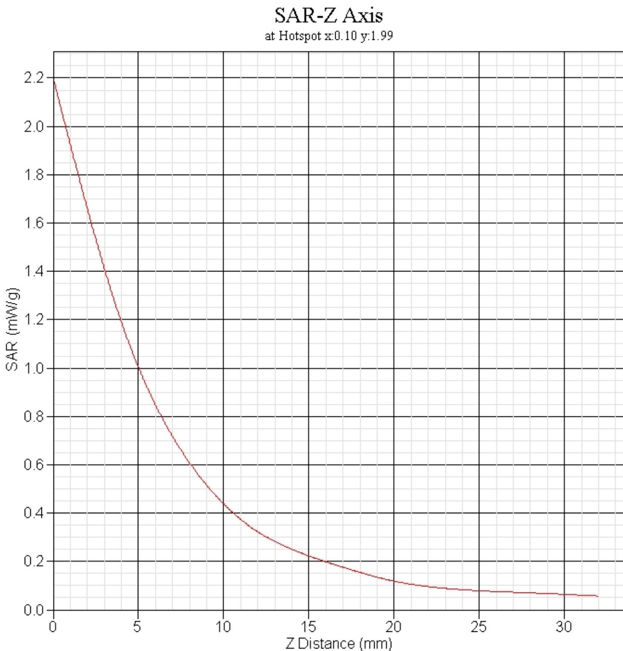
**EUT 2450MHz SAR test Z-Axis plot****(802.11g, Rear, Channel 1)**
