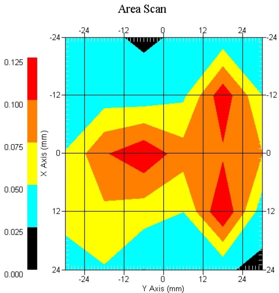
**EUT 2450MHz SAR test Z-Axis plot****(802.11b, Rear, Channel 1)**
