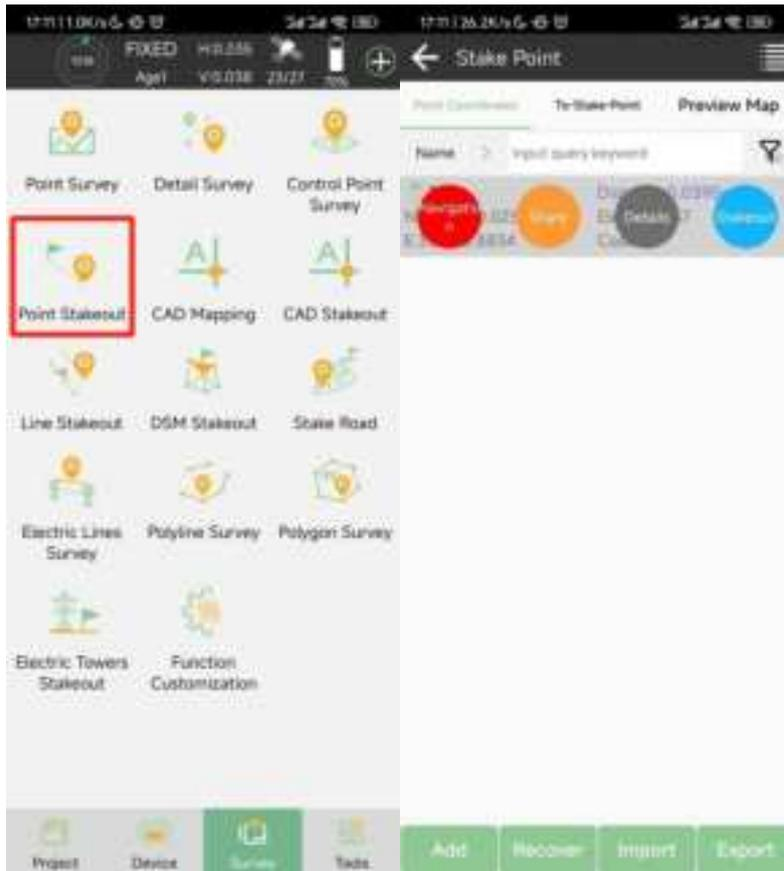
Choose a point to stake, SingularPad provides a navigation map when staking points/lines. If you are close to the target point enough, it will alarm you based on the alarm range you set.
