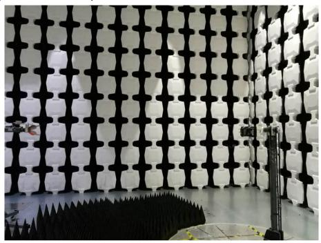
Description: Substitution Antenna for EIRP Test
