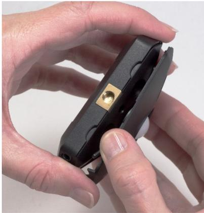
Insert the Batteries. Insert two (2) AAA batteries as shown. Be sure to observe the polarities.
