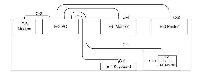
C-1 USB Cable C-2 Centronics Cable C-3 RS-232 Cable C-4 Video Cable C-5 Data Cable
