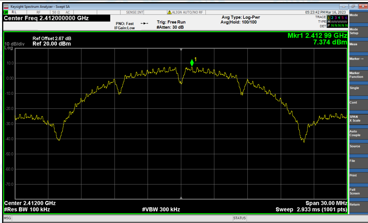
Band Edge NVNT b 2412MHz Ant1 Emission
