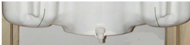
Figure 7.2 SAM Twin Phantom shell
