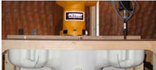
Figure 5.1 SAM Twin Phantom
