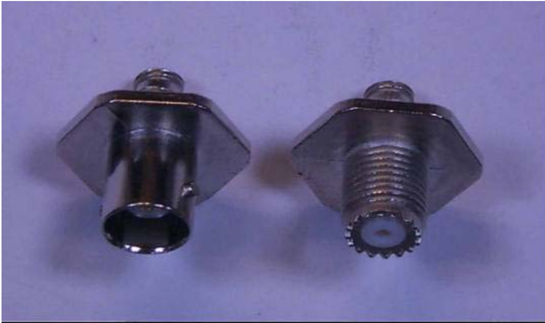
Figure 3-9: Antenna connector options, BNC (left), mini-UHF (right).
