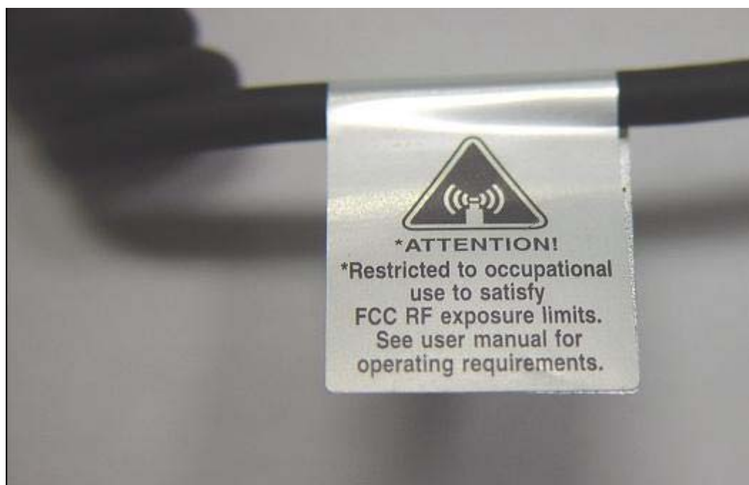
Figure 3-8: Close-Up of RF Safety Label
