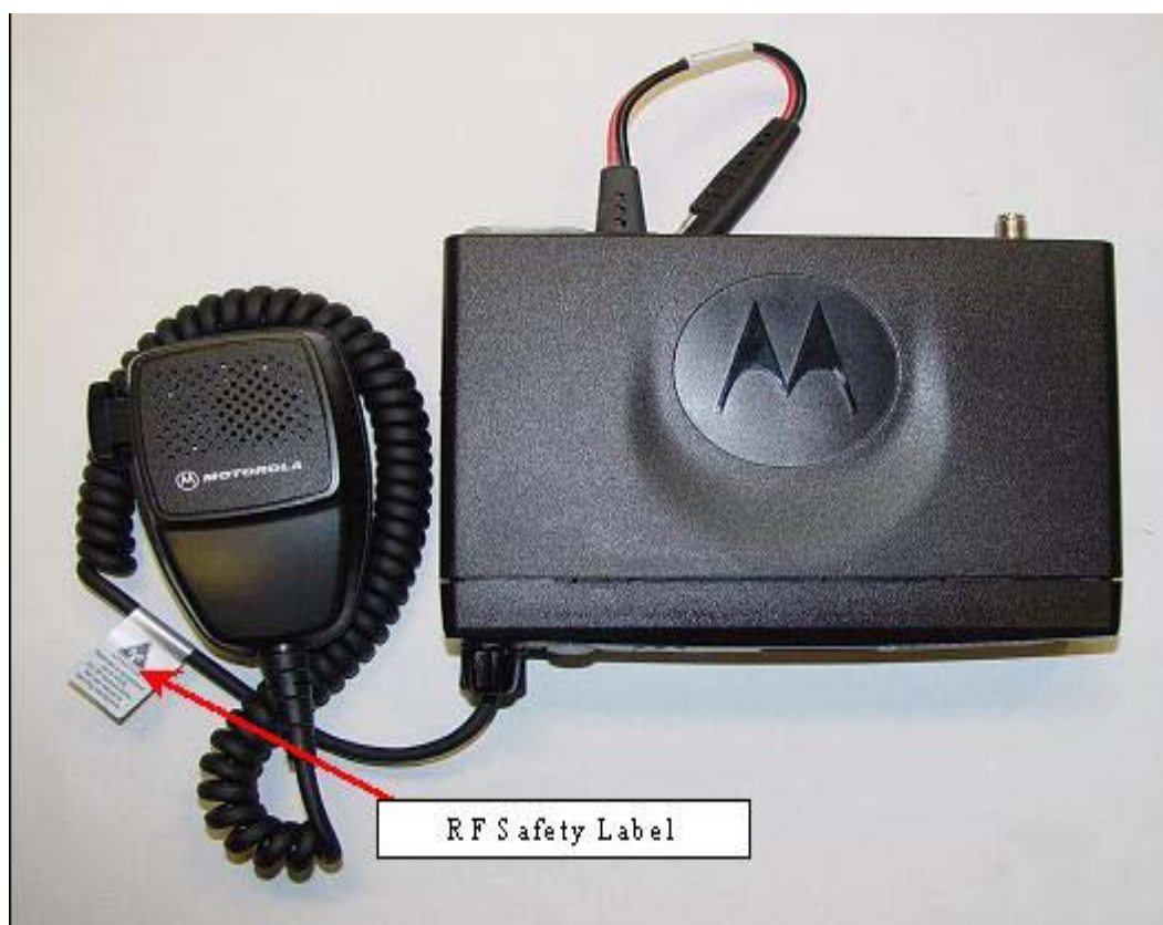
Figure 3-7: RF Safety Label Location attached to microphone cord.
