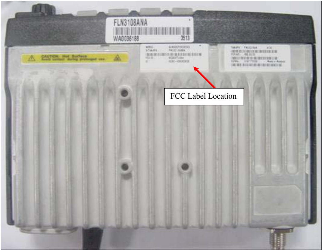
Figure 3-5: Rear View showing antenna connector, DC cable, and accessory connector.
