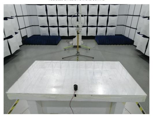
Radiated Emission 30MHz to 1000MHz
