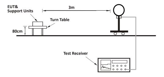
For Radiated emission 30MHz to 1GHz:
