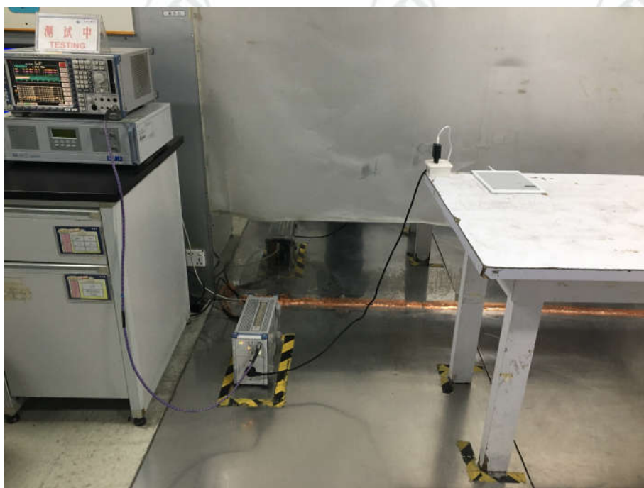
Conducted Emissions Test Setup
