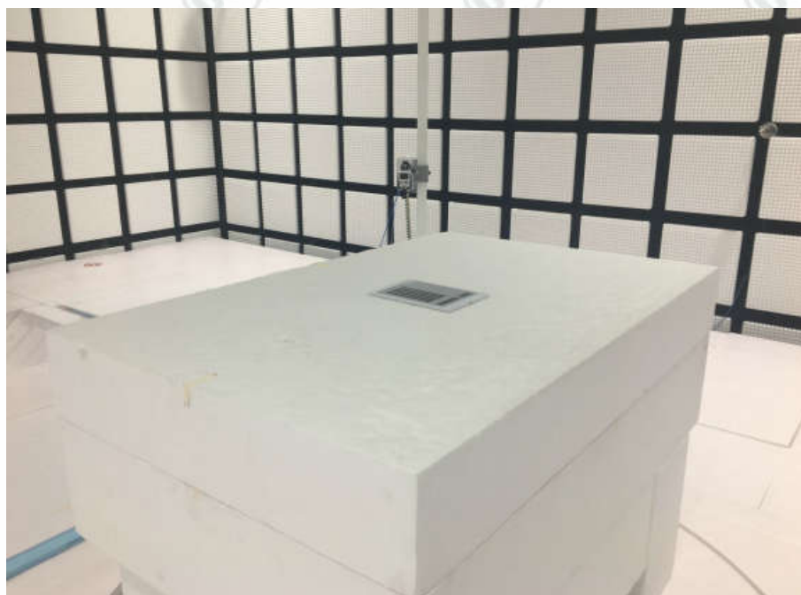
Radiated spurious emission Test Setup-4(Above 18GHz)
