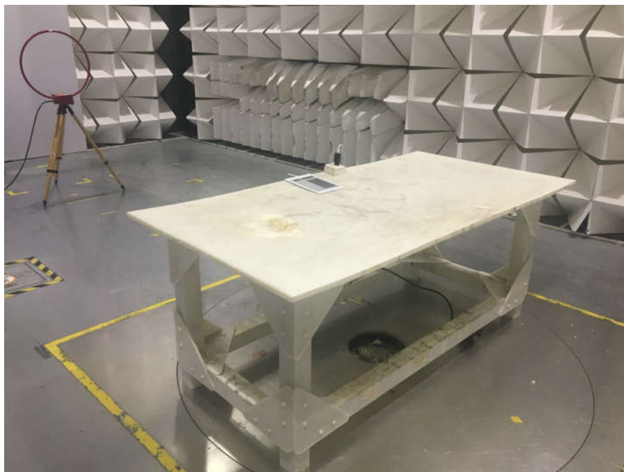
Radiated spurious emission Test Setup-1(Below 30MHz)
