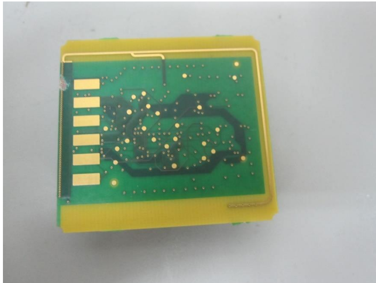
Photograph No.3 Print side of the main PCB
