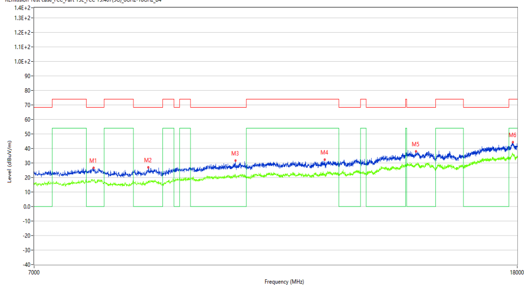
REmission Test case_FCC_Part 15E_FCC 15.407(SG)_6GHz-18GHz_B4
