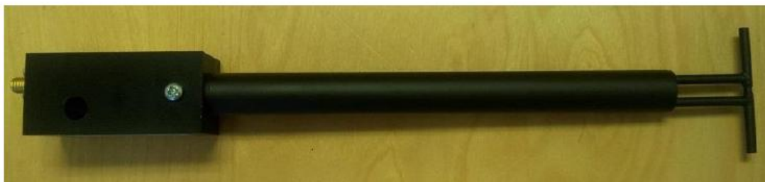
Figure 1 – MVG COMOSAR Validation Dipole
