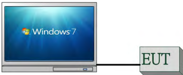
Fig. 2-2 Conducted Emission Configuration
