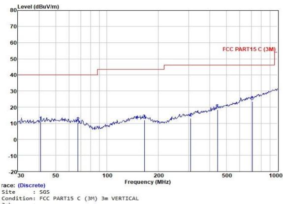
Site : SGS Condition: FCC PART15 C (3M) 3m VERTICAL Job : Model : Power : Test Mode: Right
