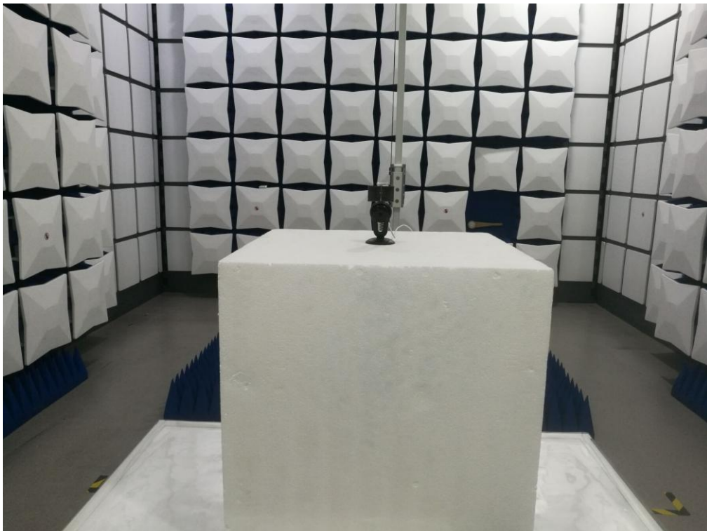
FCC RADIATED EMISSION TEST SETUP ABOVE 1GHZ
