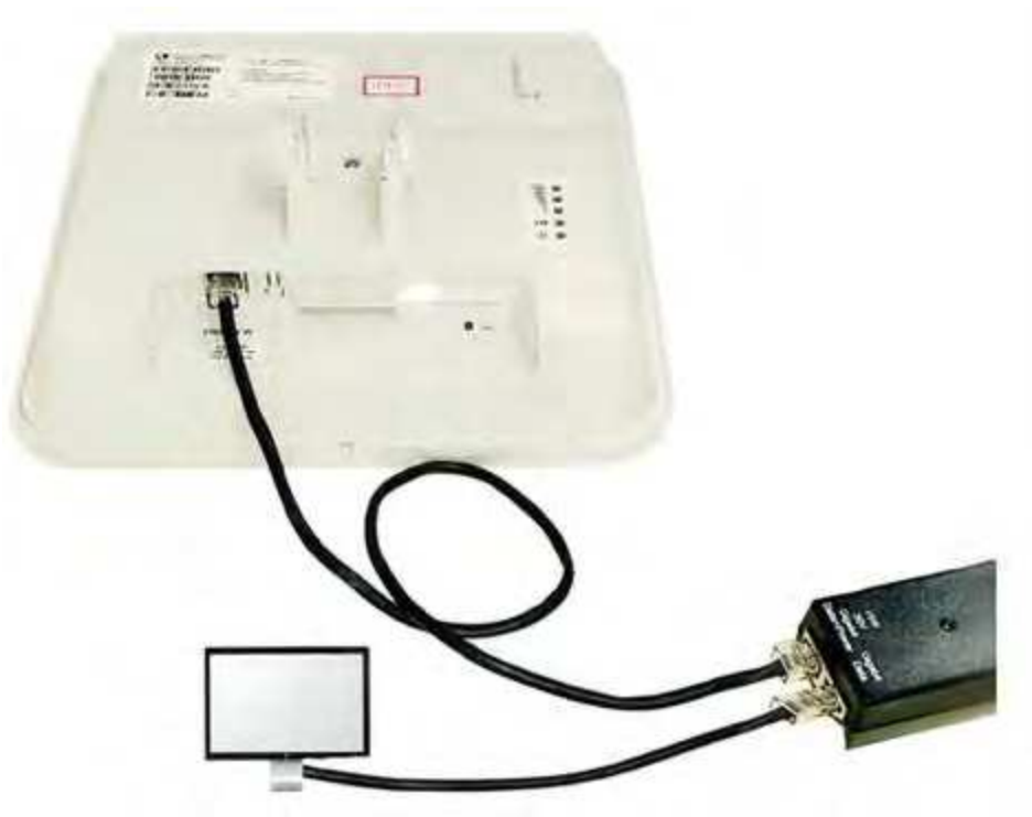
Figure 28 : Installation of Tyndall 101 to PoE adapter
