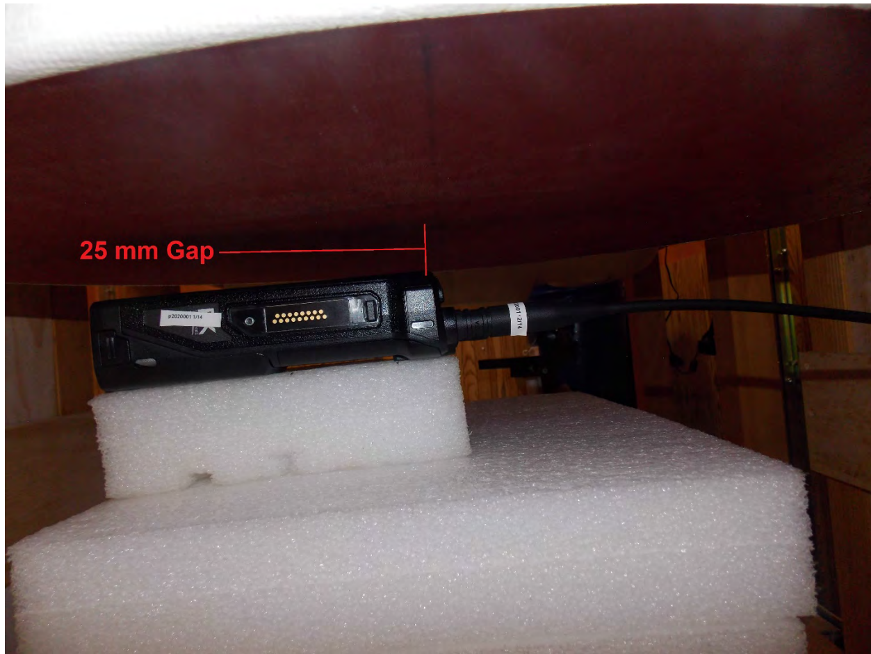
Handset Face Ant A Configuration
