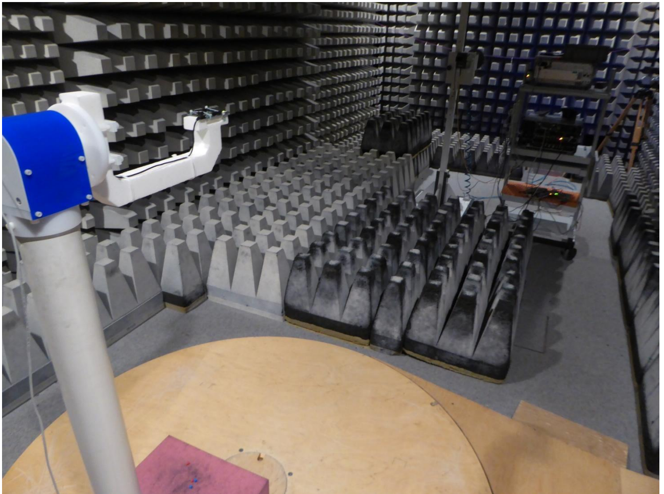
Test setup fully anechoic chamber 18 – 26.5 GHz
