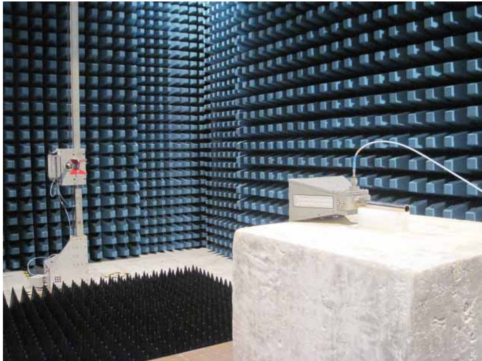
Description: Substitution Antenna for EIRP Test
