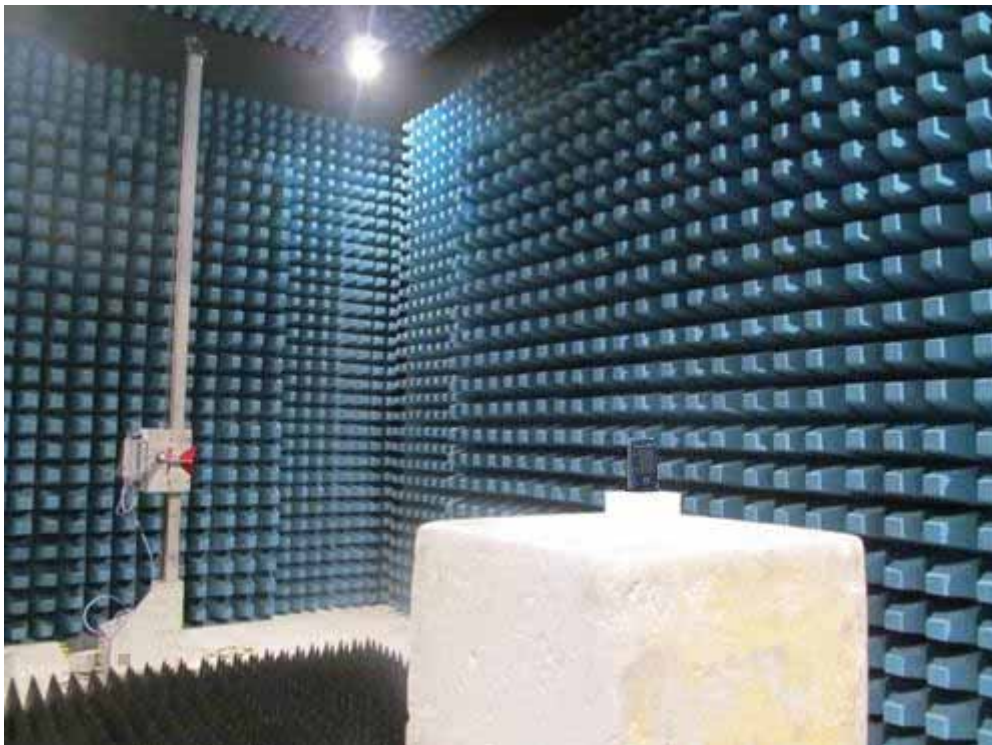
Description: EIRP Test Setup
