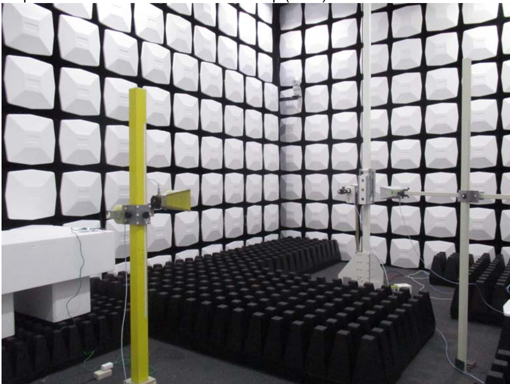
Description : Radiated Emission Test Setup (Horn)
