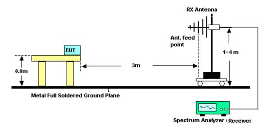
For radiated emissions from 1GHz to 18GHz
