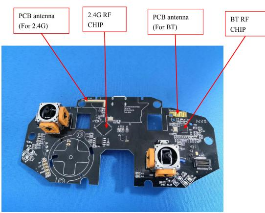
BT RF CHIP: Model :Realtek8761 2.4G RF CHIP: Model :DN2406U Manufacturer:Realtek
