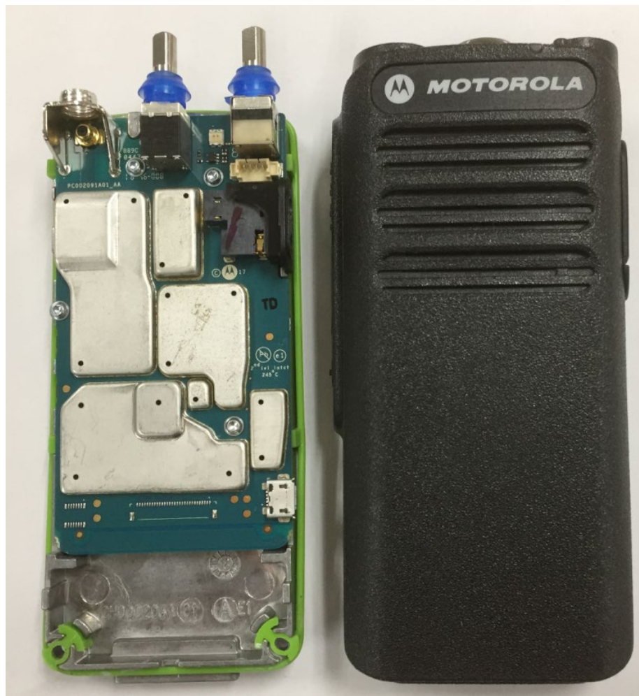
RF board with chassis and housing (front side)
