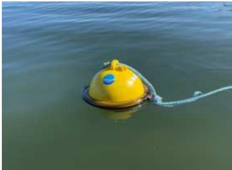
Figure 4: Smart buoy correct orientation while floating.
