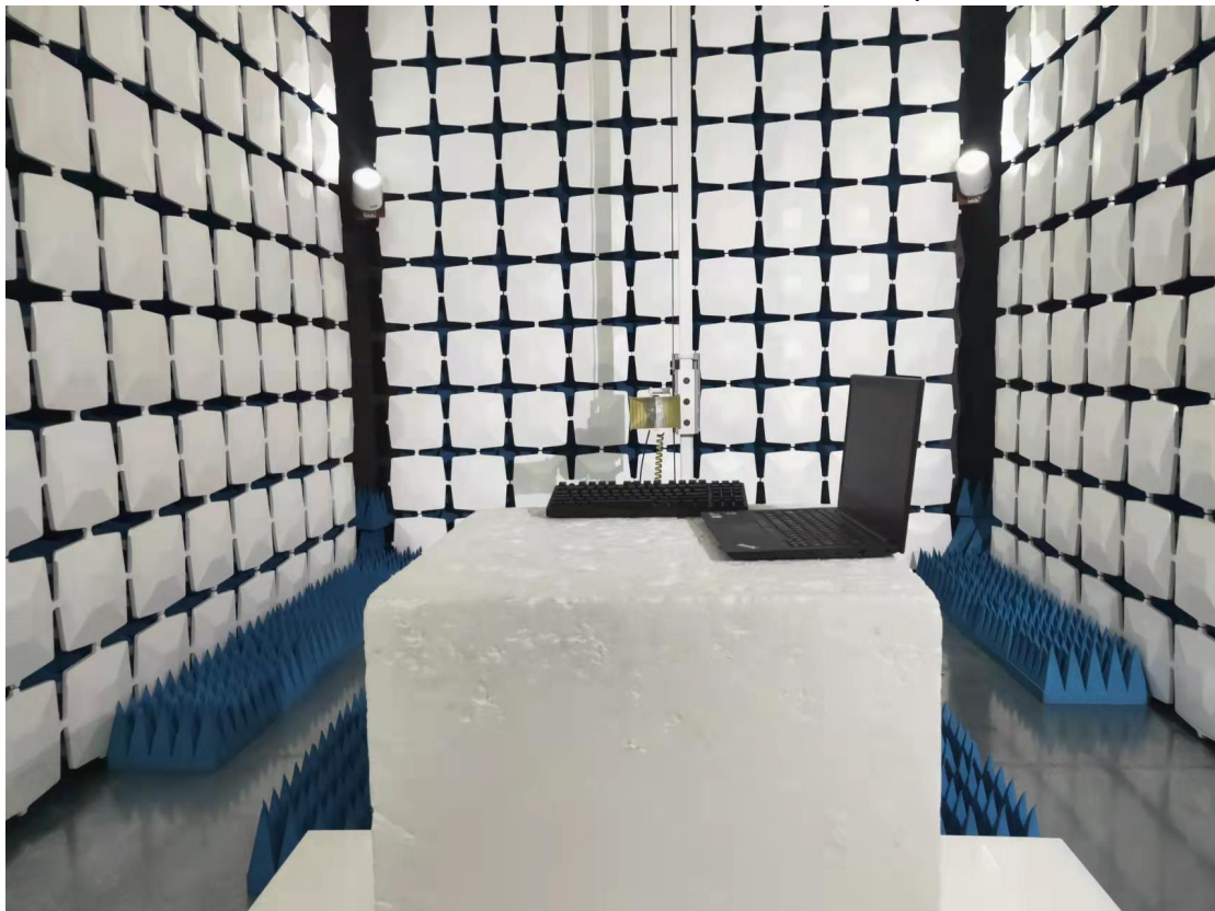
Above 1GHz for radiated emission test setup
